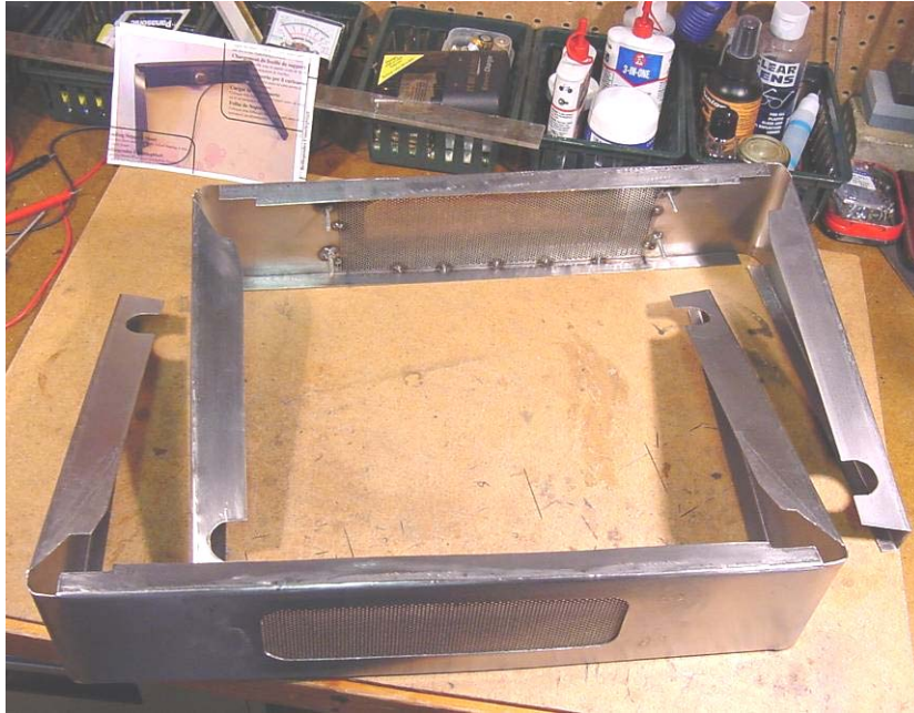
Above: Both of my replica Type 906 plinths under construction - after bending and installing the perforated metal speaker grills (note photo of the prototype in background)
