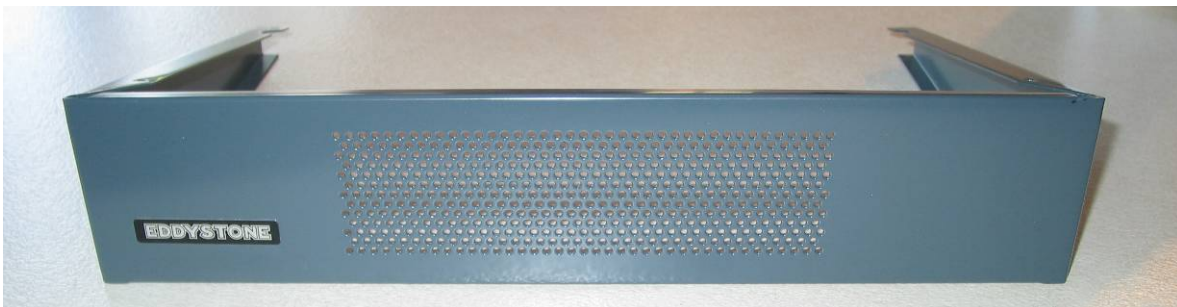
Above: One of Mike's 'clone' Type 989 plinths with the punched panel
